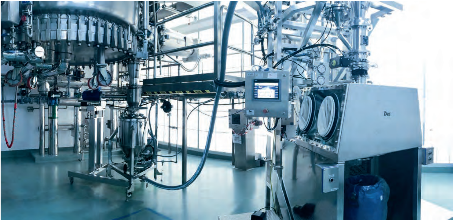
High Containment Pack-Off (patented technology) Filling solution for drums after a process, in this case filterdrying and milling. Eliminates the need of a clean room.
