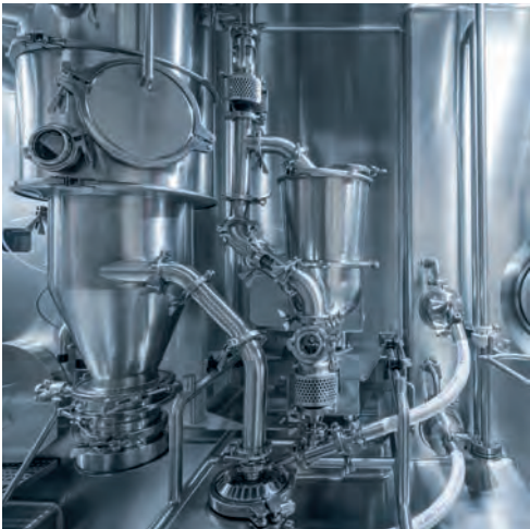
Micronizing and milling chamber with MC DecJet® interchangeable jet mills and mechanical mill
