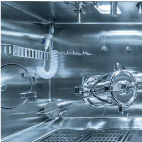
Multipurpose chamber designed for dispensing and Tubular® blending or post-conditioning at low temperature on trays with RH control
