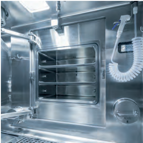
Post-Conditioning Chamber High temperature and RH conditioning through-the-wall chamber
