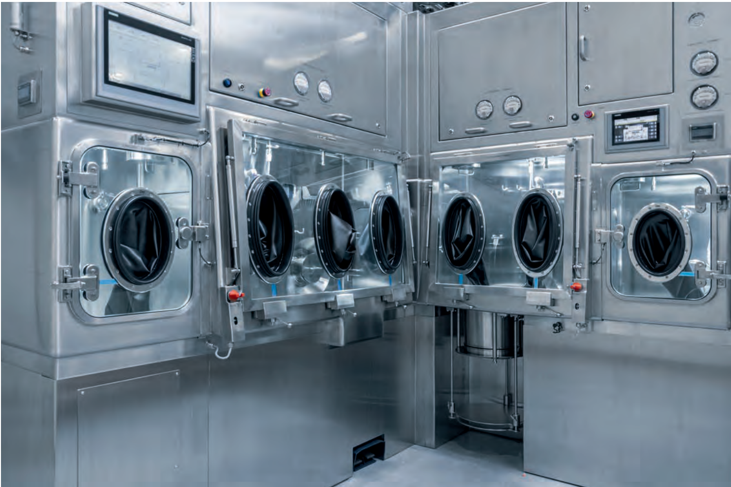
High Containment System for Milling, Micronizing, Dispensing, Sampling, Blending, and Post-Conditioning
