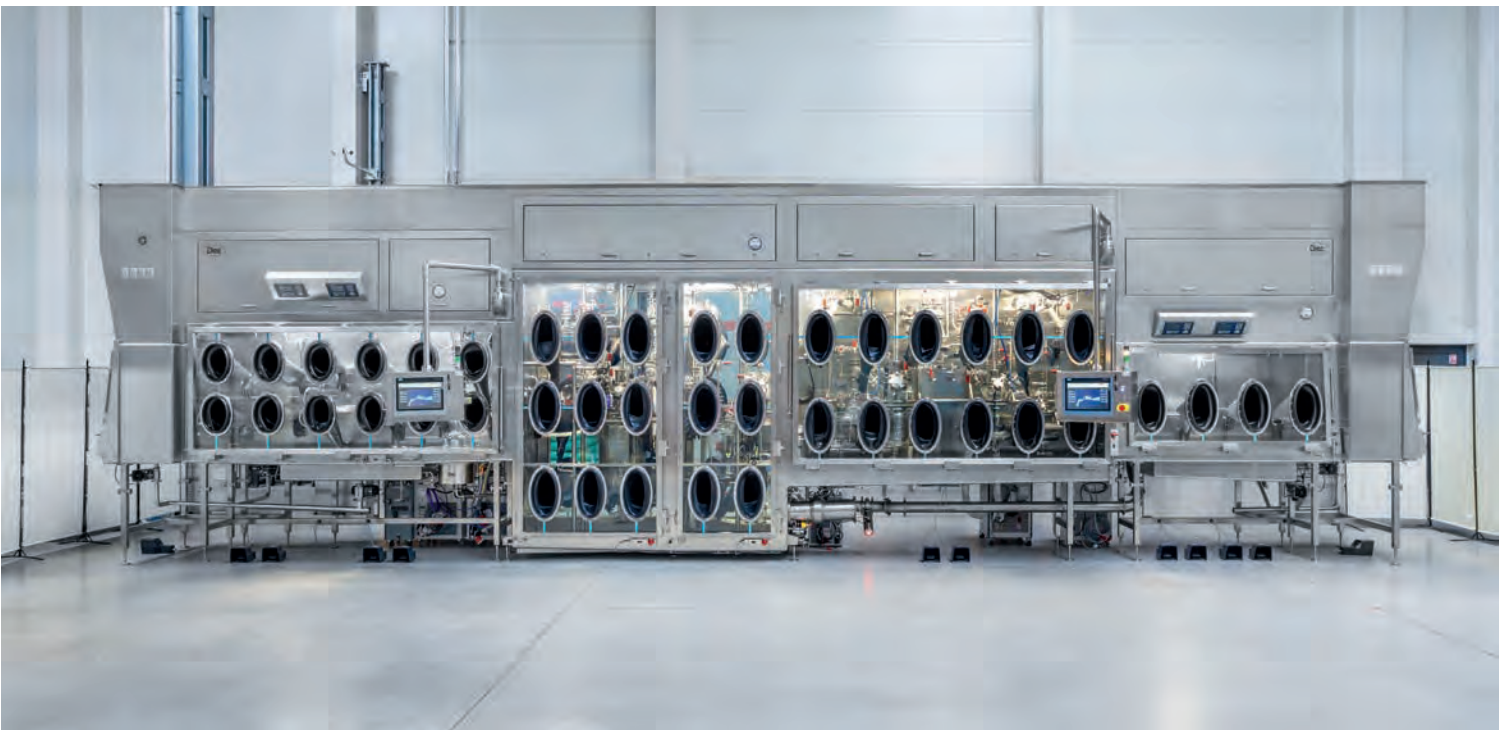
Isolator for Antibody-Drug Conjugates (ADC) targeted therapy manufacturing Reaction, filtration and Vacuum Drying
