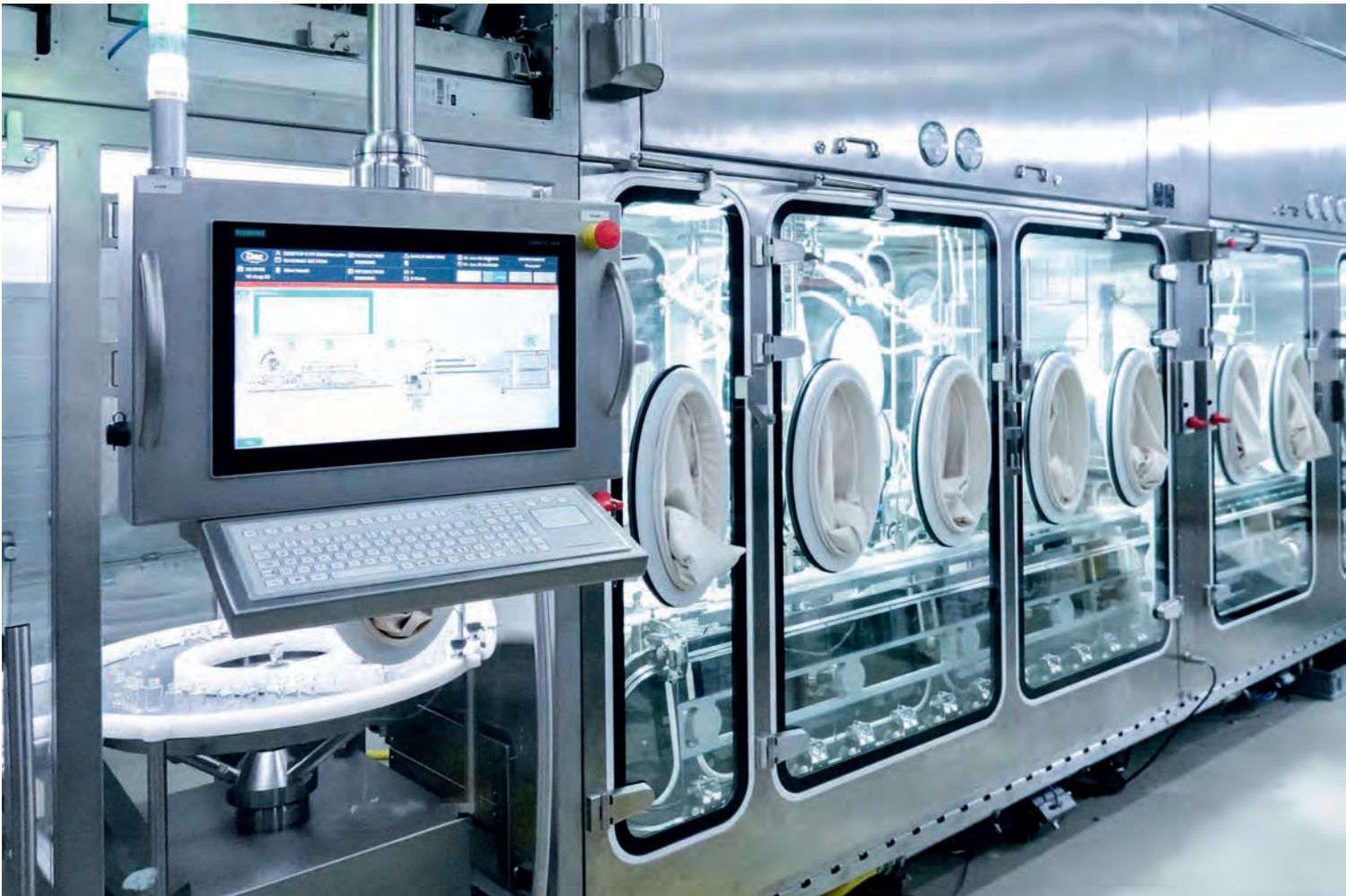
Aseptic Filling Line Fully automated and modular production scale fill-finish operation
