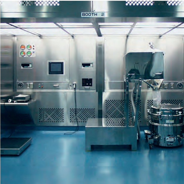
Downflow booth with integrated weighing and dispensing equipment
