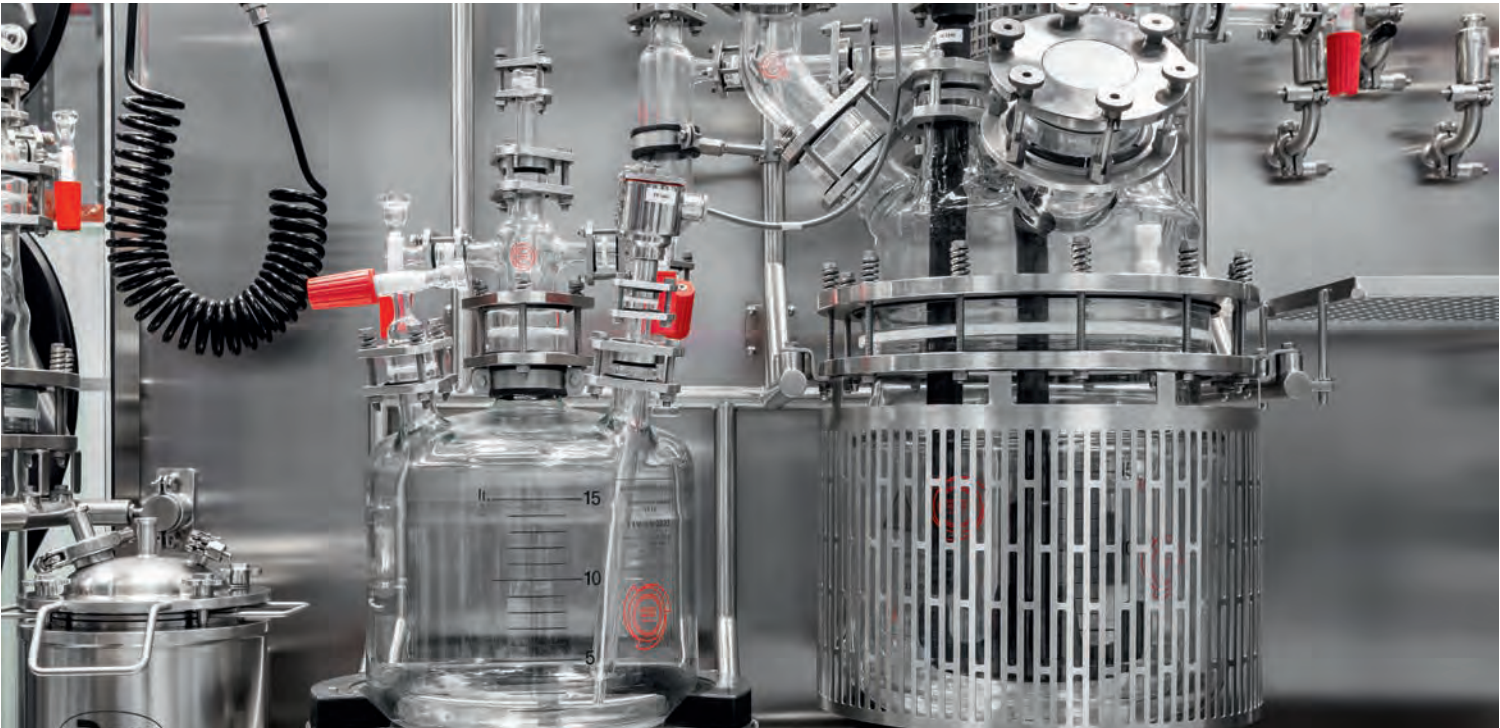
Wet Process Chamber Integrated small scale glass reactors
