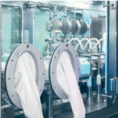
Open and Closed RABS (Restricted Access Barrier System) to provide a controlled environment for aseptic processing and sterile drug filling
