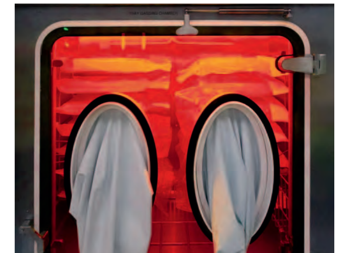
VHP decontamination: Fast Gassing Airlock integrated design for tray offloading
