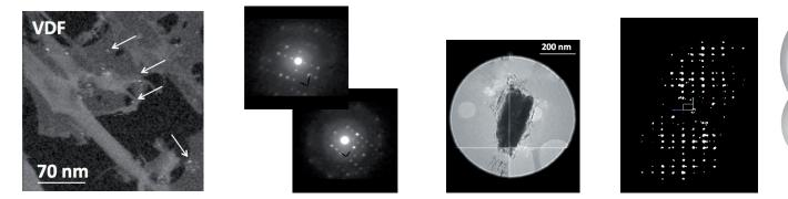
From left to right : Virtual Dark Field (VDF) TEM high resolution image showing 10 nm resorcinol crystals (arrows) on amorphous background; corresponding ED patterns for crystallites; individual Nicotinic acid API nanocrystal and its corresponding ED pattern
