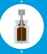
**FILLING** – The exact amount of filling as measured by the dosing system is fed into the container via the mandrel.
