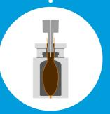
**BLOWING** – The mould closes and, in doing so, welds the base. The mandrel is positioned on the neck of the container and blows sterile air into the parison to create the desired shape. Small containers are created using a vacuum.
