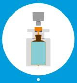
**SEALING** – Once the mandrel is removed, the head mould comes together to form the desired closure type.
