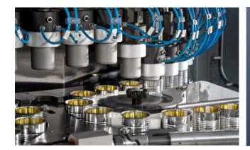
Bonfiglioli Engineering offers customized solutions from 100 ml up to 1000 ml in filled cans and up to 30 liters in empty cans and 100 to 600 containers per minute in filled cans and up to 1200
