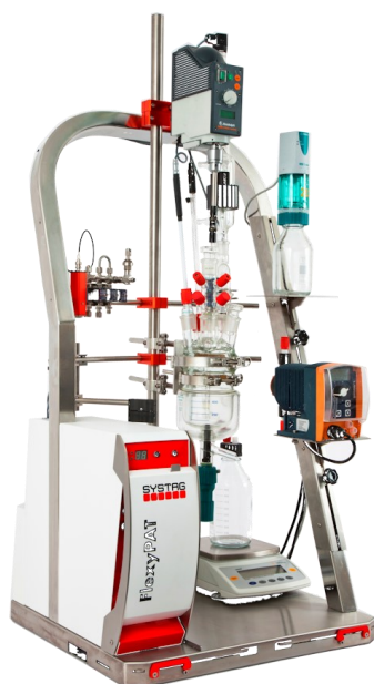
Chart 1: FlexyPAT Heat flow calorimeter
