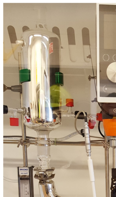
Chart 2: Special reflux cooler for heat balance method
