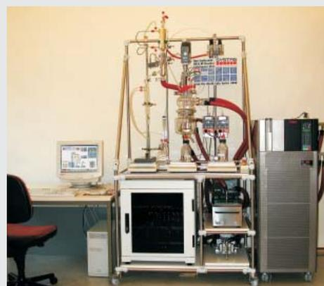
Calo2310 eco or Calo2310 base can be directly assembled into a desk mounted hood (only upper frame structure).
