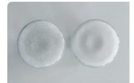
Figure 2: Lyophilisate structures of a 5% saccharose solution, for comparison: left SynchroFreeze – right standard
