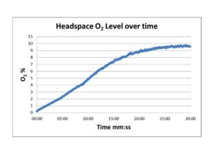
Headspace oxygen increase in vial with laser drilled hole of 5 µm equivalent diameter from the moment of stoppering.\*
