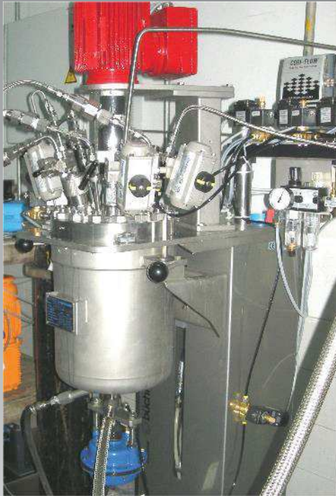
3lt. / 100 bar reactor / Ethylene feed / autom. bottom valve / Ex-compliant
