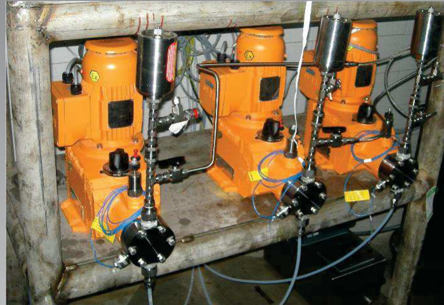
High pressure pumps up to 60 bar, pulsation free feeding, ex-proof
