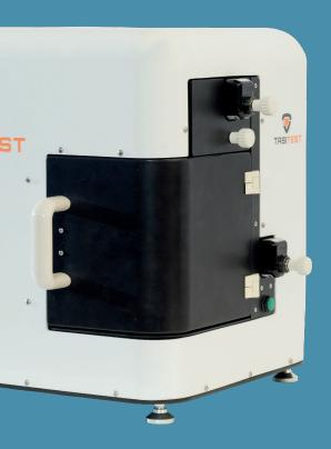
It is a non-destructive, non-invasive laser-based inspection technology for measuring the headspace levels of gases, such as oxygen and carbon dioxide, as well as monitoring moisture levels.
