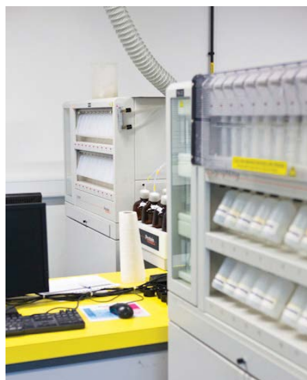
Fig. 7: Synthesizer, fully automated machine for solid phase peptide synthesis. The left picture shows reactors in which synthesis is already proceeding.
