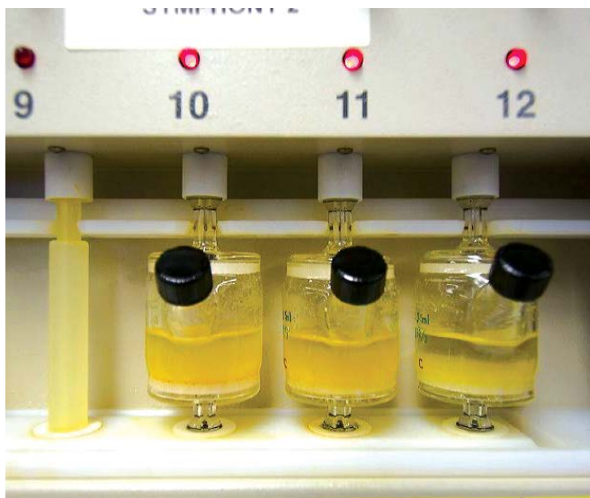
Fig. 7: Synthesizer, fully automated machine for solid phase peptide synthesis. The left picture shows reactors in which synthesis is already proceeding.
