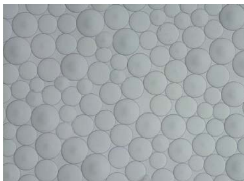
Fig. 8: Swollen resin beads under the microscope.
