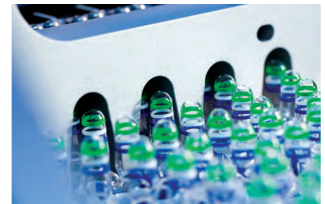
Ampoule Infeed Standing Ampoules are delivered via a feeding table to the pick and place handling units
