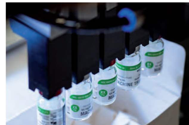
Standing Vial Insertion Vials are inserted into the open carton via pick and place handling stations
