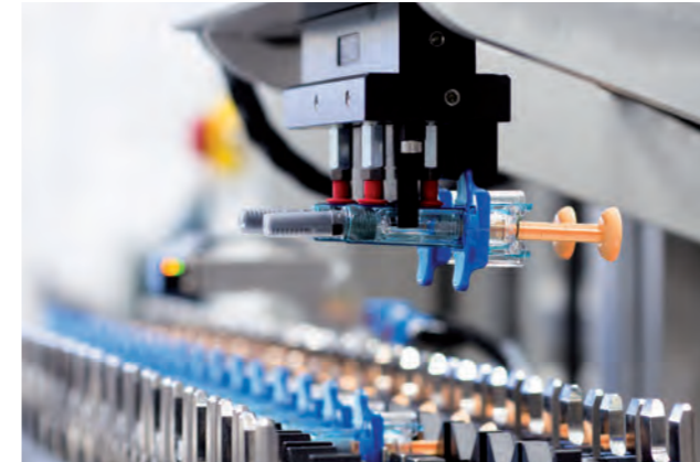
Prefilled Syringe Inserter The Syringes are delivered lying down through a PUCK system
