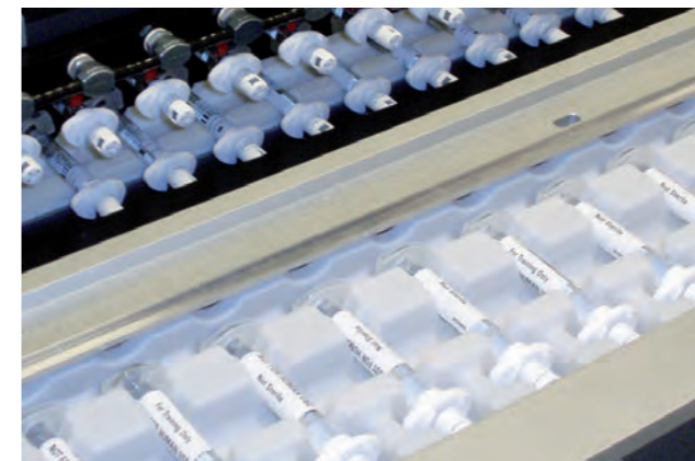
Syringes in trays Syringes are delivered to the inserting station in trays
