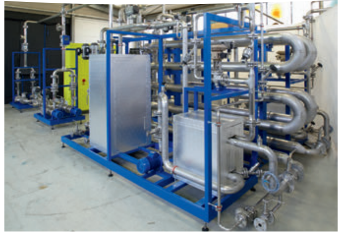
SteriFix E15000 (max. 15000 L/h, 80°C, 80 sec.) at Merck Serono GmbH for factory acceptance test
