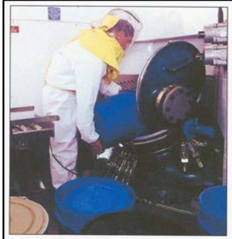
Powder charging through an open manhole
