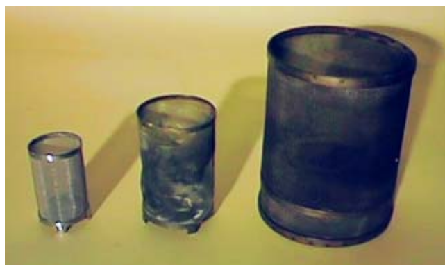
From left to right: simple wire baskets for different filling quantities for a self-heating test in SEDEX.
