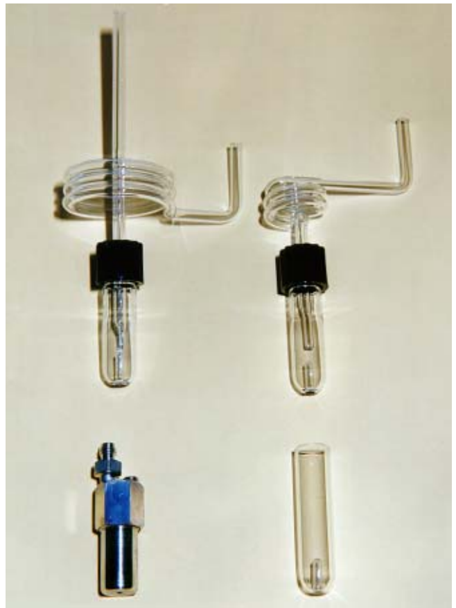
Clockwise from top left: gassed glass vessel with output measurement, standard gassing, pressure vessel with bursting foils or bursting screw (30, 100 and 200 bar models), open glass vessel, all vessels approx. 3 ml (standard filling 2.5 ml).
