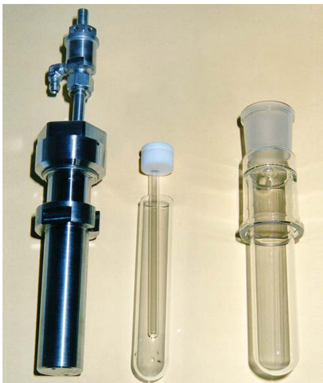
From left to right: pressure vessel with 150 bar bursting disk, glass liner for pressure vessel, Pt-100 glass liner and PTFE lid, open glass vessel with standard taper-ground joint.
