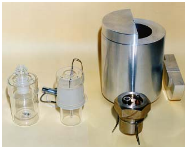
From left to right: double jacket vessel with magnetic stirrer rod, single jacket vessel with glass liner for Pt-100, 150 bar pressure vessel (front), adiabatic stabilising compartments for special experiments over very long times (back).
