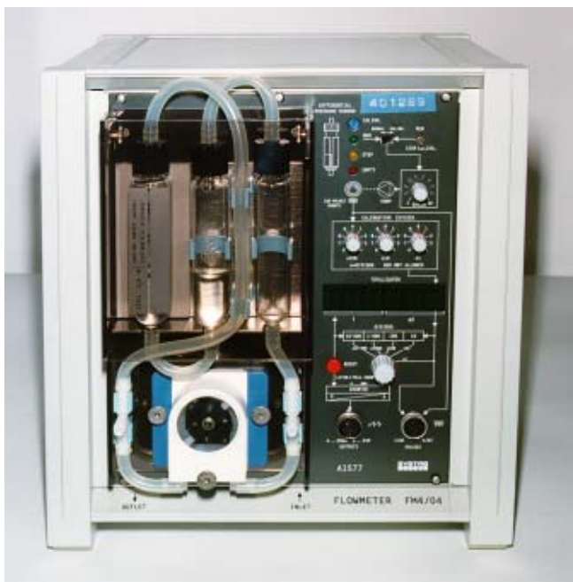
Gas flow meter FM4 for the smallest gas fluids with extremely low back pressure (approx. 1 .. 2 mbar). Measurement range FM4/4: 4l/h or FM4/60: 60 l/h. Has its application with all RADEX, RADEX V5, SEDEX and SIKAREX systems.
