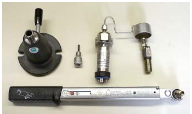
Clockwise from top left: collet attachment (tool part) with pressure vessel (bottom part), torque wrench inset for bursting screw, pressure transmitter with connection parts and pressure vessel, torque wrench with pressure vessel cover (second part of assembling tool).
