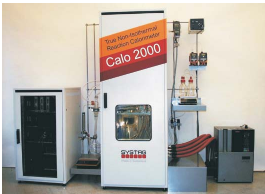
Calo 2100 with Tango for limited temperature range 0 - 100^{\circ}\text{C}
