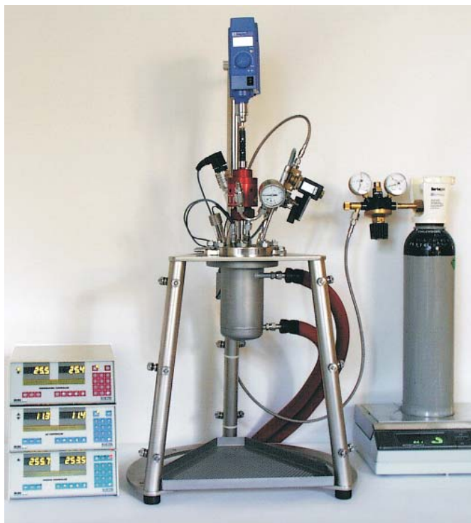
SysCalo SC1 with gas dosage, 60 bar
