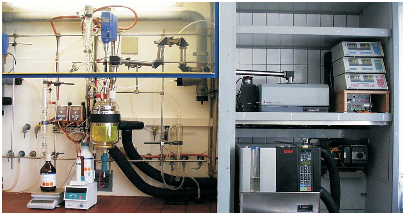
SysCalo SC2 with FTIR and pH option, as low temperature (-85°C) version
