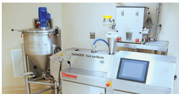
The advantages of the Twin Screw Granulator are a continuous process, limited upscaling problems and the absence of solvents.
