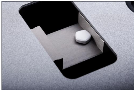
→ Tablet sample oriented in hardness measuring station of MultiTest 50
